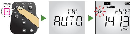
4. Press ENT button to confirm the conductivity reading. To abort calibration, press MEAS key.
