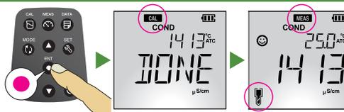
5. Repeat step nos. 1 to 4 to perform calibration with the next standard solution(s).
