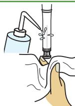
2. Immerse the conductivity electrode in standard solution.
