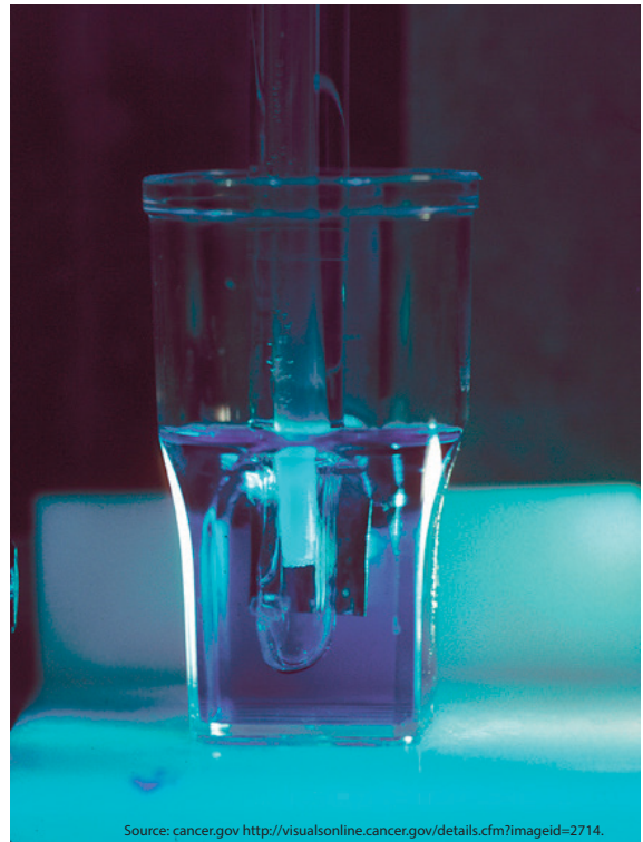
The Coulter Counter, shown here counting cells in solution, is an indirect volumetric particle analysis method.
