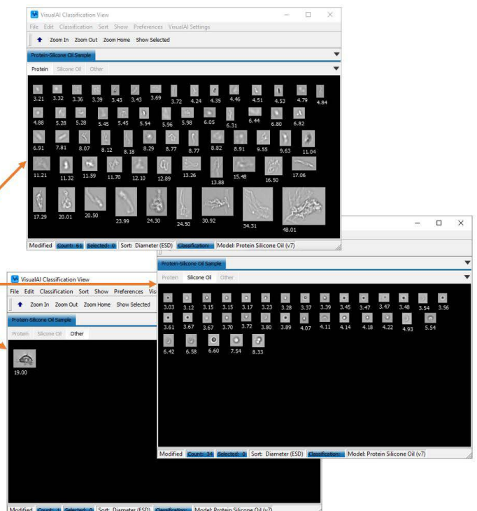
Figure 2. The graphical user interface of VisualAI. (Left) Sample FIM image collage from a sample containing 50% protein aggregates 50% silicone oil droplets. This sample was prepared as described by this study. (Right) Collages in VisualAI’s graphical user interface showing the images identified by AI utilities that contain (top) protein aggregates, (middle) silicone oil droplets, and (bottom) other particles.
