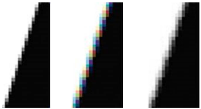
Figure 2. Simulated edge artifacts when imaging a sharp edge using a grayscale camera (left) and a color camera (center). Also shown is the color image of the edge cast to grayscale (right).
