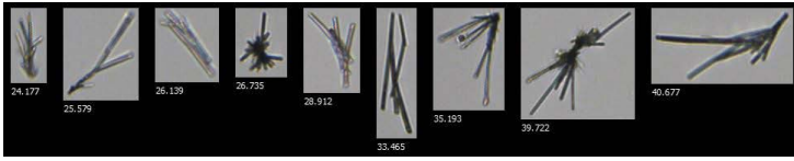
Figure 3: Example images of FDA precipitate found in the pond sample that also fluoresce green. These particles can be auto-selected using VisualSpreadsheet's image recognition algorithm to produce accurate concentrations of live cells.
