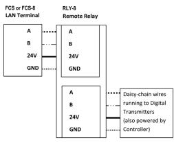
The RLY-8 can be wired directly to the FCS or FCS-8 followed by digital transmitters connected in a daisy-chain configuration. Or it can be wired anywhere along the digital network in a daisy-chain configuration as required.
