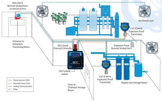
Inside the oil extraction processing area, a CXT-A-IC4H10 Explosion Proof transmitter with an infrared Butane sensor should be mounted 6 inches from the floor near the extractor and where the gas is likely to collect. Butane is heavier than air and will collect in low places. Outside the door of the extraction processing area door should be an audible/visual alarm device such as the RSH-24-R Remote Strobe / Horn.
