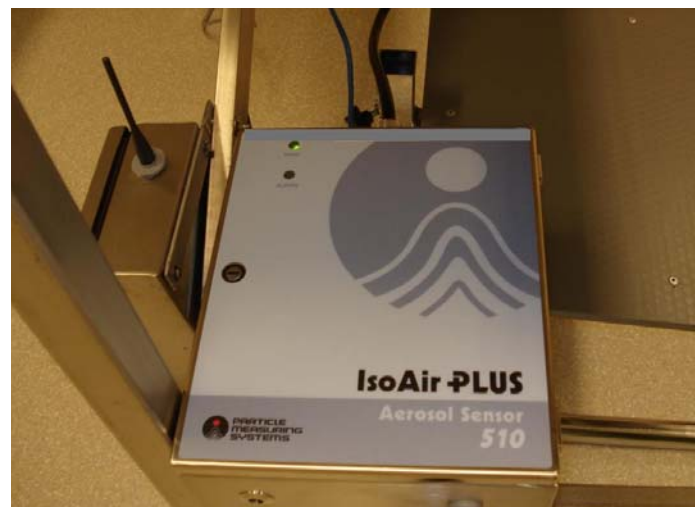
Figure 1. Particle Sensor with built-in pump and wireless communication.
