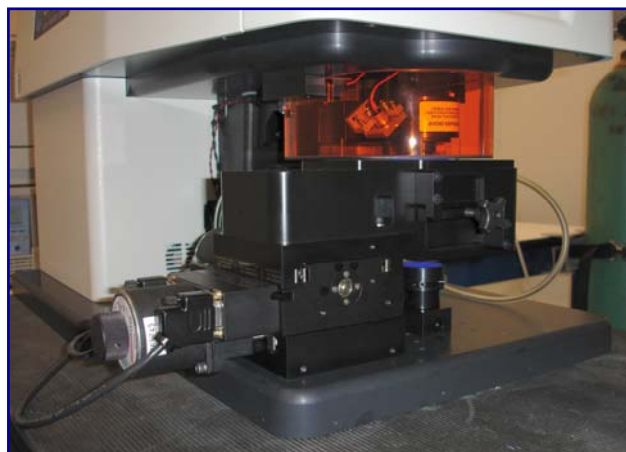
Figure 2: SuperCell installed onto the Universal Platform stage Switching from the standard cell to the SuperCell™ is completed in < 5 minutes. This can be accomplished without changing the state (shutting off) the Spectrometer's ICP.
