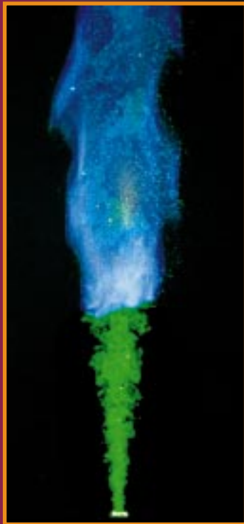
Mie scattering from a lifted jet flame. Courtesy: Stanford University
